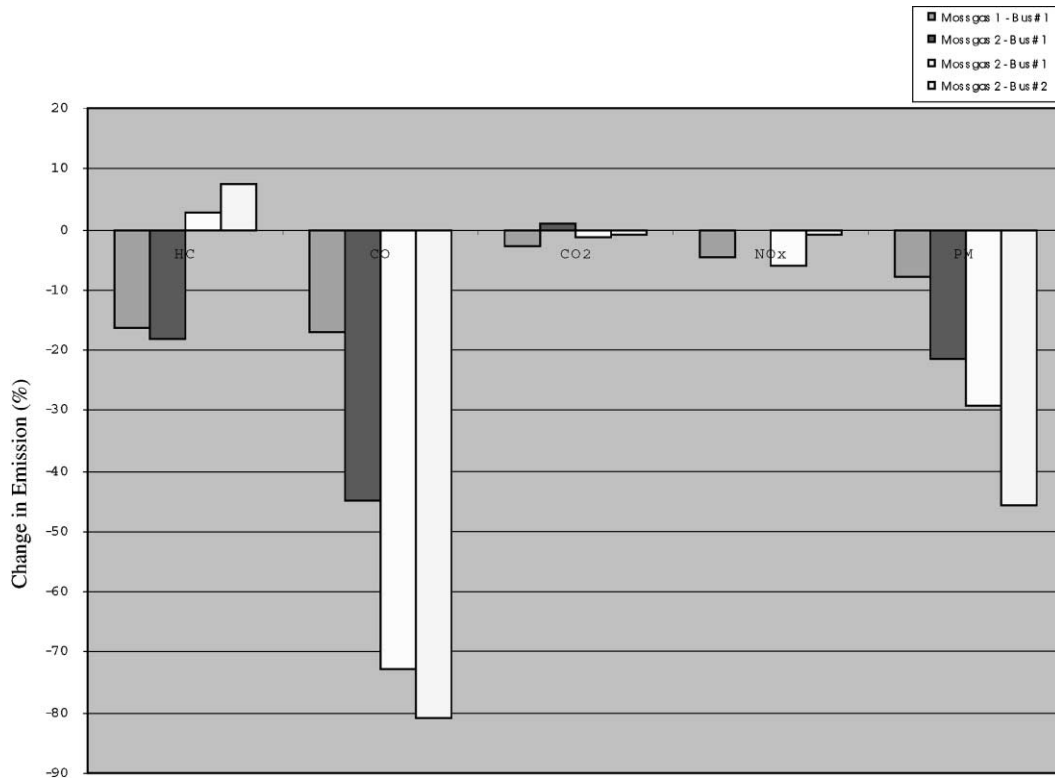
Fig. 3. Emission increase—reductions over D2 fuel catalytically equipped bus versus non-modified bus as tested over the CBD bus cycle.
